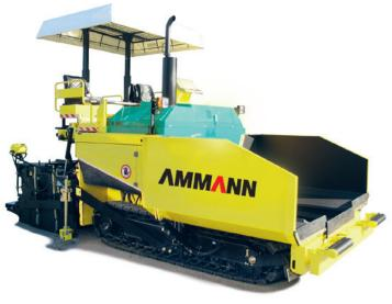
Tracked machine with rubber pads; automatic tensioning device system with grease accumulator. Hydrostatic transmission with two variable flow rate pumps which feed two motors with two displacements directly fastened to the planetary gearboxes which operate the tracks. Mounted on each pump, an electronic and proportional control gives a progressive start and stop,
